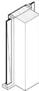
Figure 5.6: 3D detail of the façade connection on the load-bearing structure: external insulation 15
